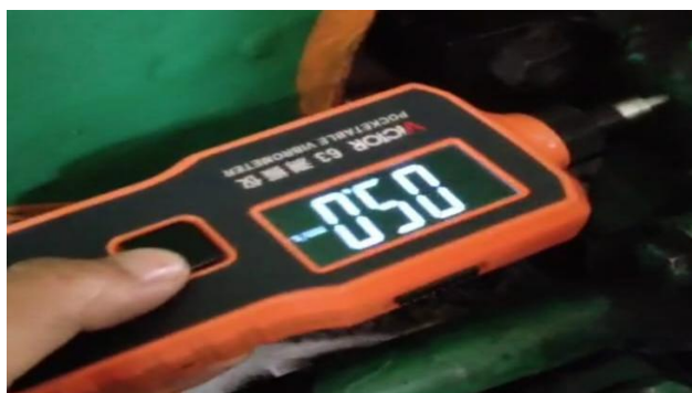
Gambar 4.2 Pengukuran Vibrasi Bearing 1 Horizontal B
