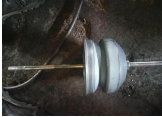
Gambar 2.17 Steam Valve (Adibrata Unggul Jaya)
