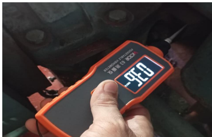
Gambar 4.4 Pengukuran Vibrasi Bearing 1 Arah Aksial
