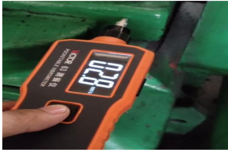
Gambar 4.16 Pengukuran Vibrasi Bearing 2 Horizontal B
