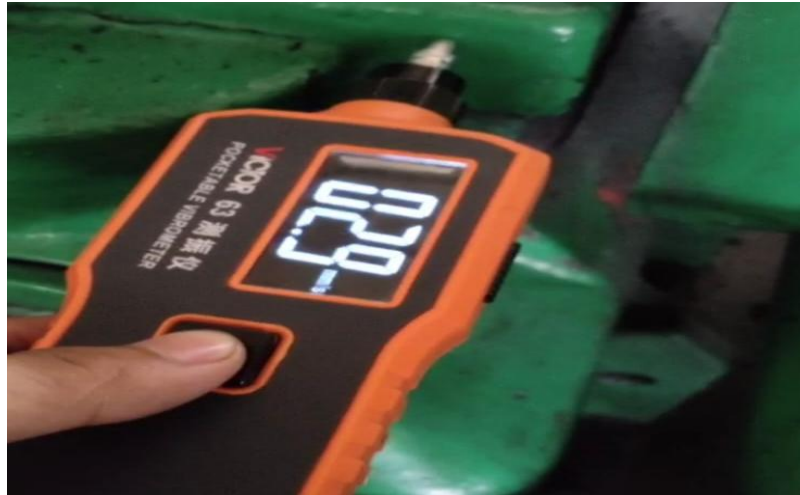
Gambar 4.12 Pengukuran Vibrasi Bearing 1 Horizontal B
