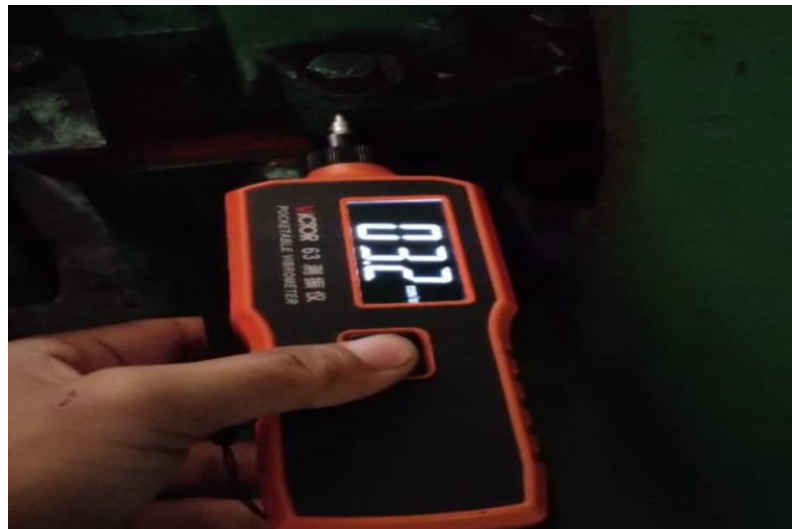
Gambar 4.15 Pengukuran Vibrasi Bearing 2 Horizontal A
