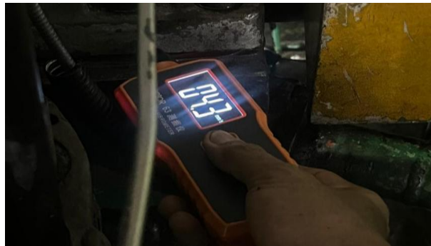
Gambar 4.1 Pengukuran Vibrasi Bearing 1 Horizontal A
