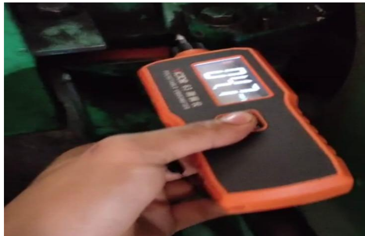
Gambar 4.6 Pengukuran Vibrasi Bearing 2 Arah Horizontal B
