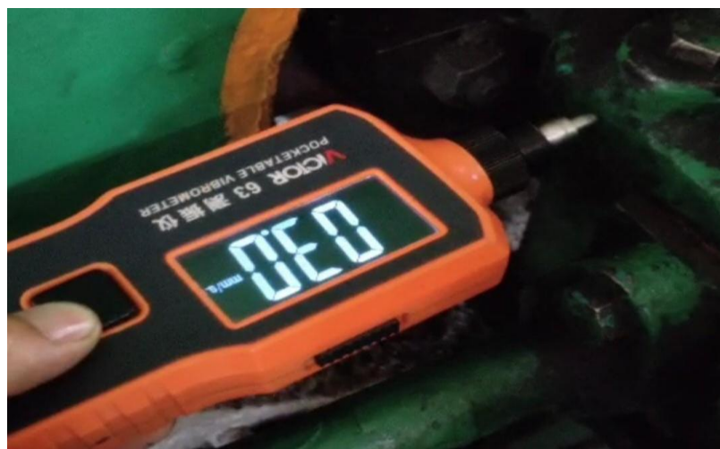
Gambar 4.11 Pengukuran Vibrasi Bearing 1 Horizontal A
