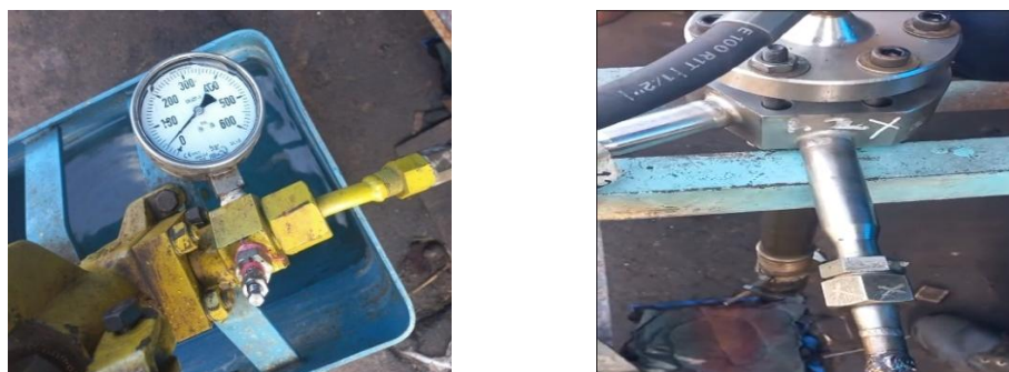
Gambar 4.18 Inspeksi Fuel Nozzle Spray Test
