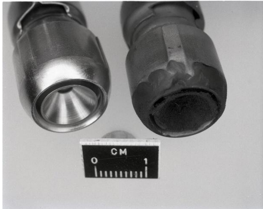
Gambar 2. 3 Fuel Nozzle Mengalami Carbon Deposit
