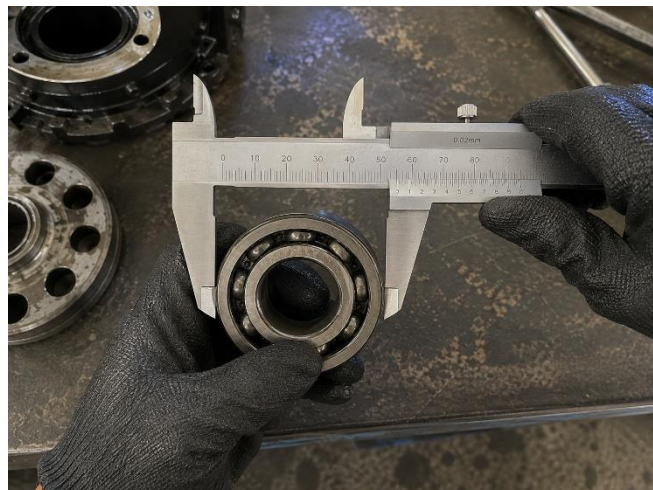
Gambar 4.7 pengukuran diameter bearing .
