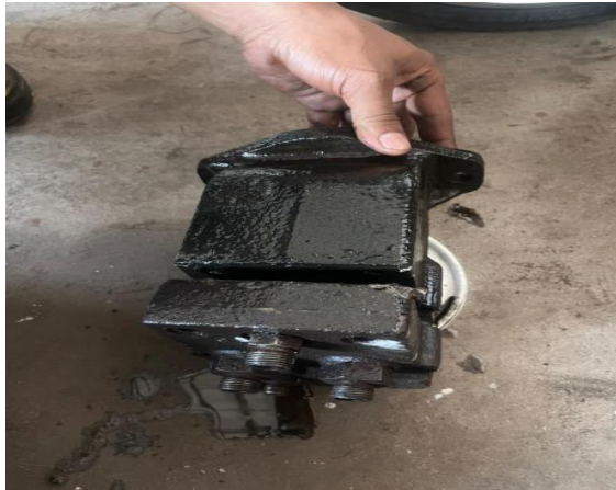
Gambar 3.1 Motor Drive Hidraulik
