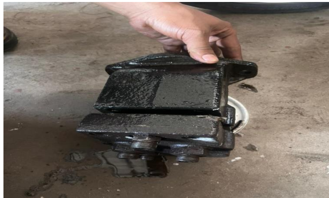
Gambar 2.3 Housing (Casing Motor)
