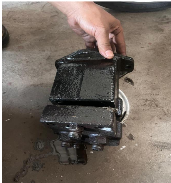
Gambar 4.2 Pelepasan housing (casing motor)
