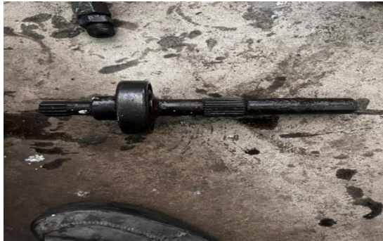
Gambar 2.5 Poros Output ( Output Shaft )
