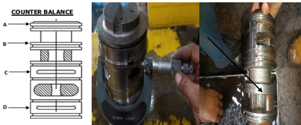
Gambar 4.8 Pengukuran Shaft Counter Balance
