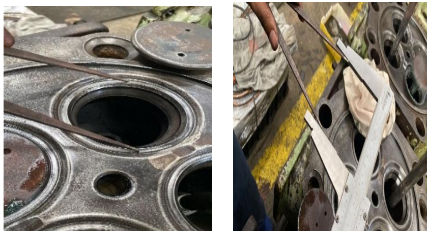
Gambar 4. 3 Pengukuran Valve Seat intake diameter luar
