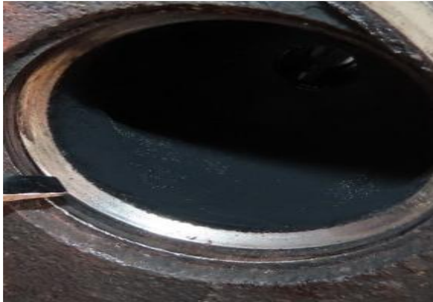
Gambar 2. 13 Keausan Valve Seat (PT. Waruna Shipyard Indonesia)
