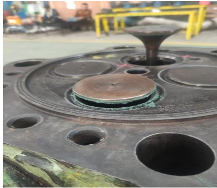
Gambar 4. 13 Penanganan kebocoran Valve Seat
