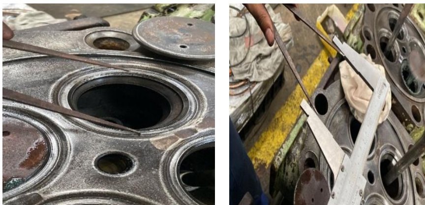
Gambar 4. 6 Pengukuran Valve Seat exhaust diameter luar
