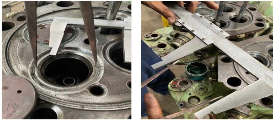
Gambar 4. 7 Pengukuran Valve Seat exhaust diameter luar
