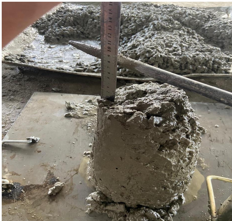
Gambar L.6: Pengujian slump test .
