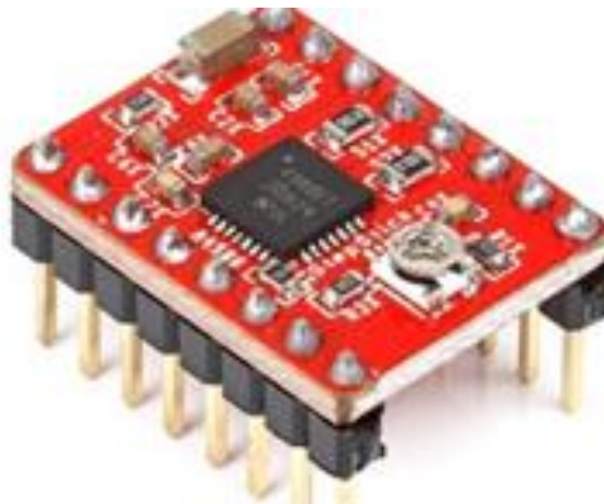
Gambar 2. 4 Motor Driver A4988
