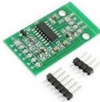
Gambar 2. 13 Modul amplifier HX711
