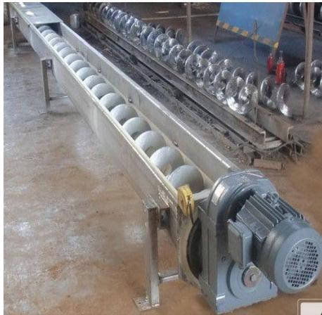
Gambar 2.2 Mesin *Screw Conveyor*
