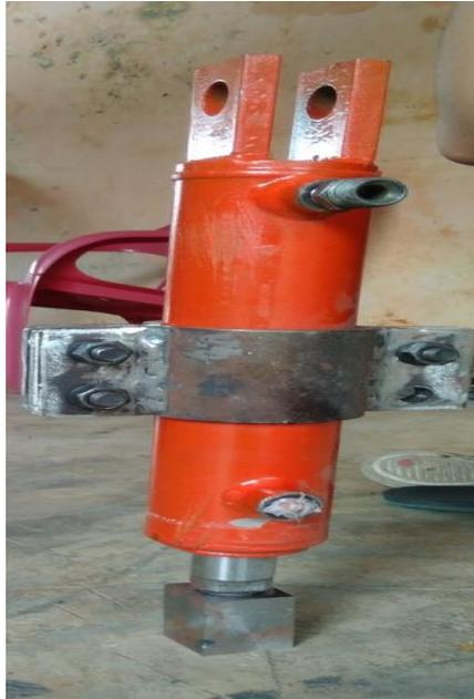
. Gambar 3.11 Aktuator ( silinder Hidrolik )
