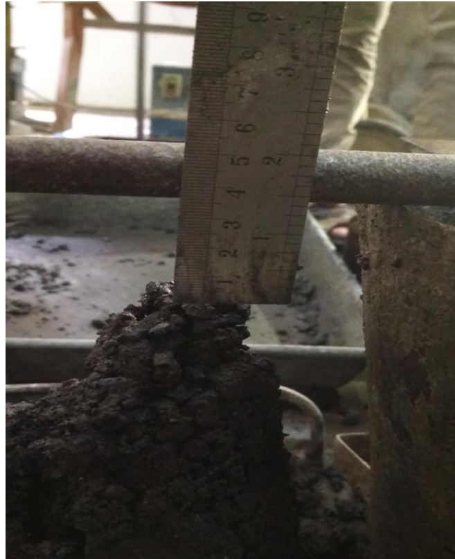
Gambar L9: Proses pengujian slump .
