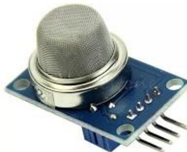
Gambar 2.1. Modul sensor gas MQ 2
