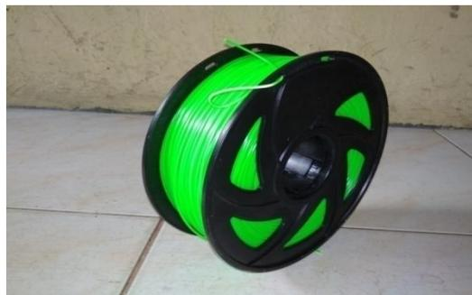
Gambar 3.4 Filament ABS (Acrylonitrile Butadiene Styrene)
