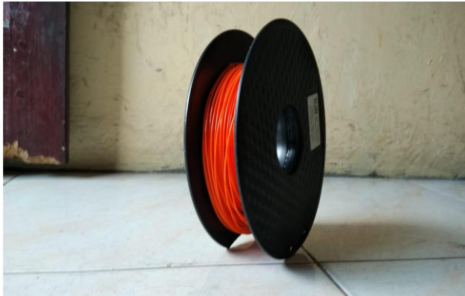
Gambar 3.4 Filament ABS (Acrylonitrile Butadiene Stryrene)
