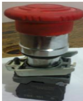
Gambar 3.11 Tombol tekan (emergency stop switch)
