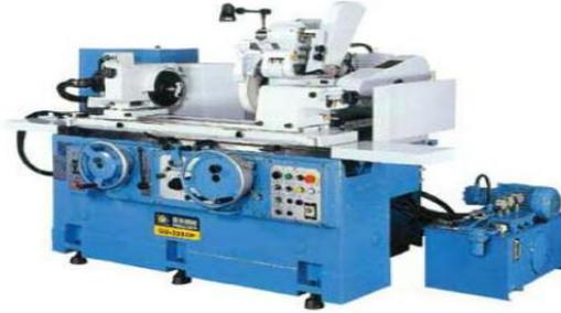
Gambar 2.5 GU 32100P *Universal Cylindrical Grinding Machine.*
