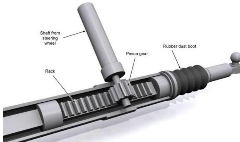
Gambar 2.13 Rack and Pinion
