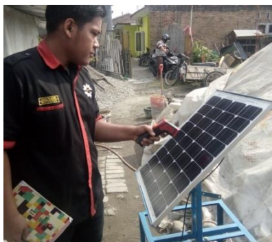
Gambar 3.32 Mengukur Temperatur Panel
