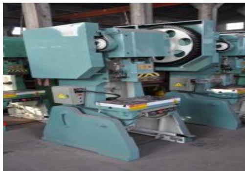
Gambar 2.3 Mesin pres mekanikal (Klikmro. 2018)
