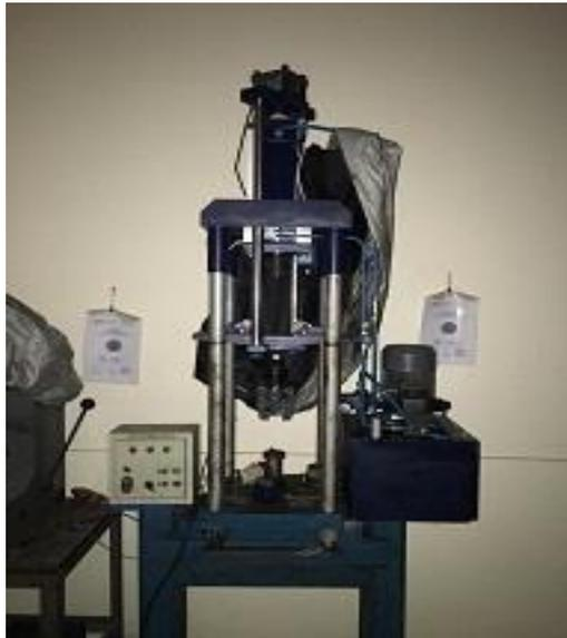
Gambar. 3.18 Alat Uji Three Point Bending
