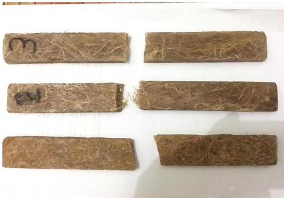
Gambar 4.4 Spesimen hasil pengujian *Three Point Bending*
