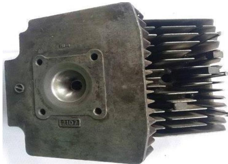
Gambar 3.5. *Cylinder Head* Motor Satria 2T
