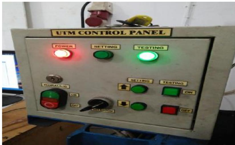
Gambar 4.16 UTM Control Panel
