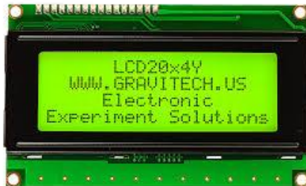
Gambar 2.9 : LCD 4x20 CHARS
