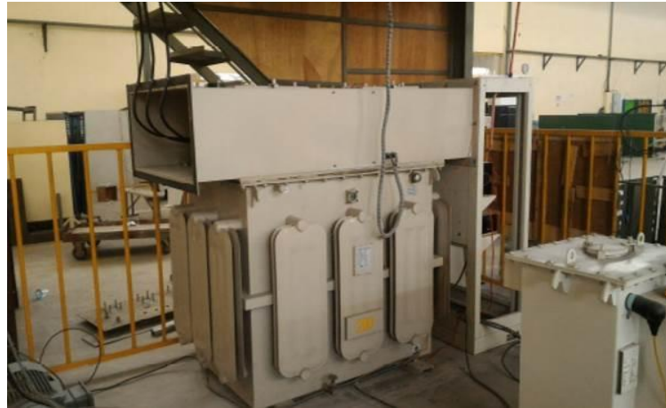
Gambar 3.1 Induction voltage regulator
