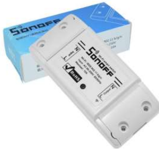
Gambar 2.1. Sonoff Wi-Fi Smart Switch
