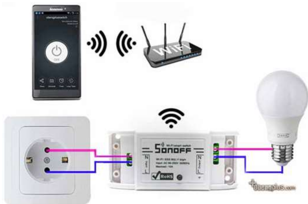
Gambar 3.1. Skema Sederhana Sonoff Wi-Fi Smart Switch
