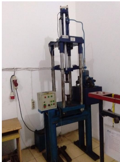
Gambar 3.8 Mesin Uji Tarik ( Universal Testing Machine )
