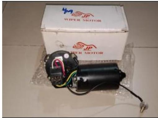
Gambar 3.14 Motor wiper dc 12v
