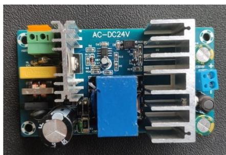
Gambar 3.10 *Adapter ac-dc 24v*
