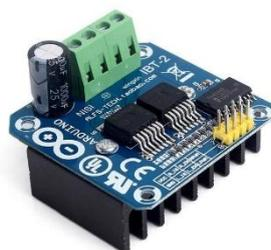
Gambar 3.13 *Driver motor bts7960b*
