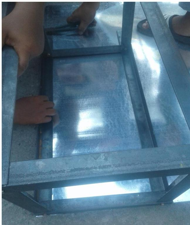
Gambar 4.4 Proses Penutupan Dinding Rangka
