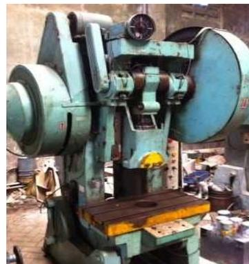
Gambar 2.3 mesin *punch* (Ach. Muhib Zainuri “Material Handling Equipment”.Cetakan pertama. Yogyakarta.Andi offset.
