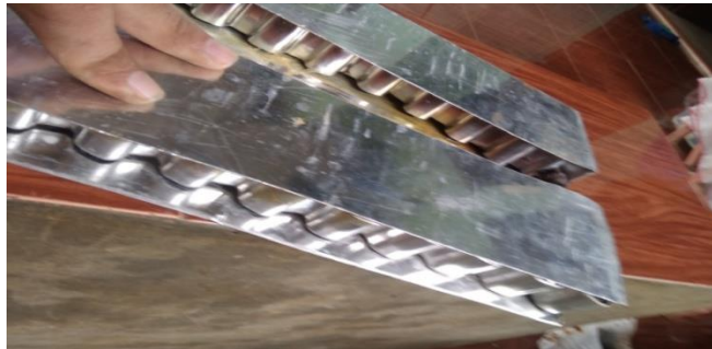
Gambar 4.16 proses penutupan struktur honeycomb
