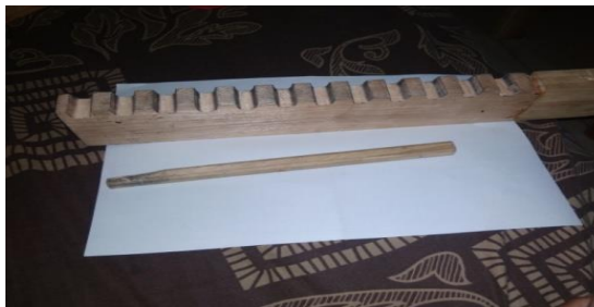
Gambar 3.2.16: Cetakan specimen ukuran sisi hexagonal 10 mm
