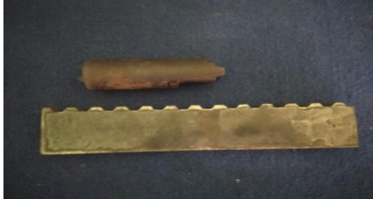
Gambar 3.2.15: Cetakan specimen ukuran sisi hexagonal 6 mm
