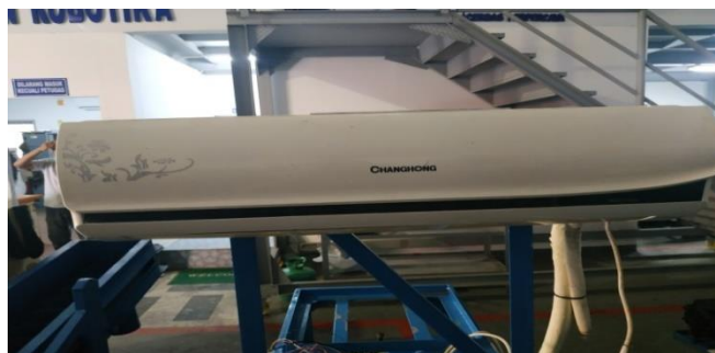
Gambar 3.2 Unit Indoor AC Split
