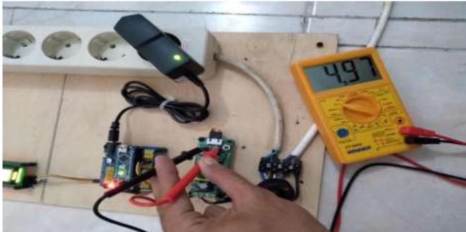
Gambar 4.3 *Output* sensor PZEM-004T
