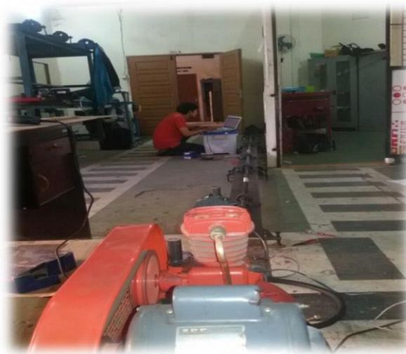
Gambar 3.10 Alat Uji Split Hopkinson Pressure Bar (SHPB)
