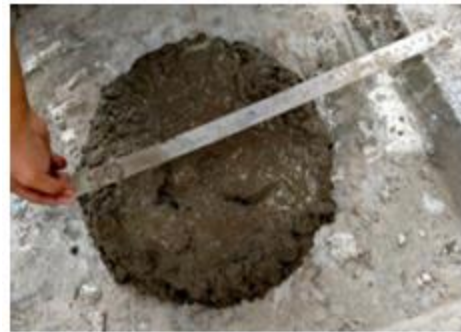
Pengujian slump flow beton SCC
