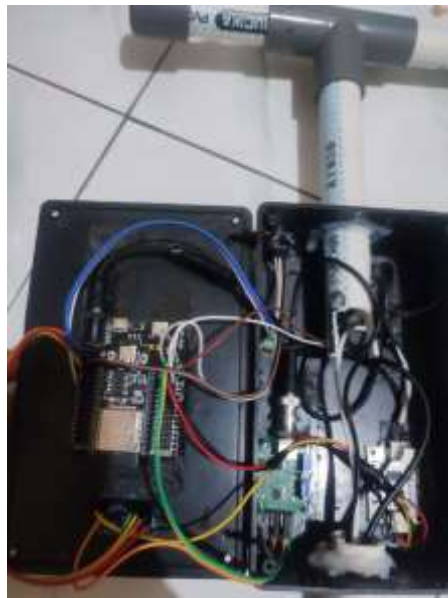
Gambar 4. 2 Detail Kompartemen Unit Kendali (IoT Box)
