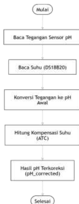
Gambar 3. 4 Diagram Alur Proses Kompensasi Suhu Otomatis (ATC)
