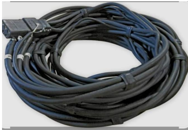
Gambar 2.2.17 Kabel Ground Power Unit
