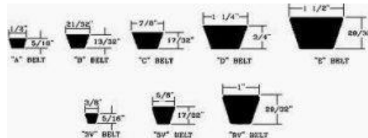
Gambar 2.10 V- Belt Standar (Sularso,1991)
