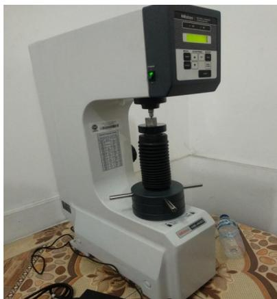
Gambar 3.11 *Hardness Rockwell test*
