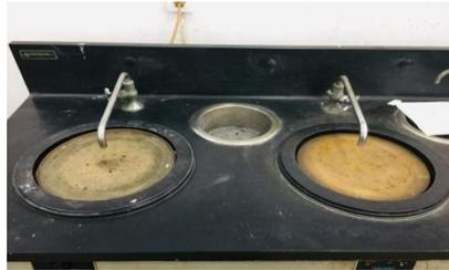
Gambar 3.22 Mesin *polishing*
