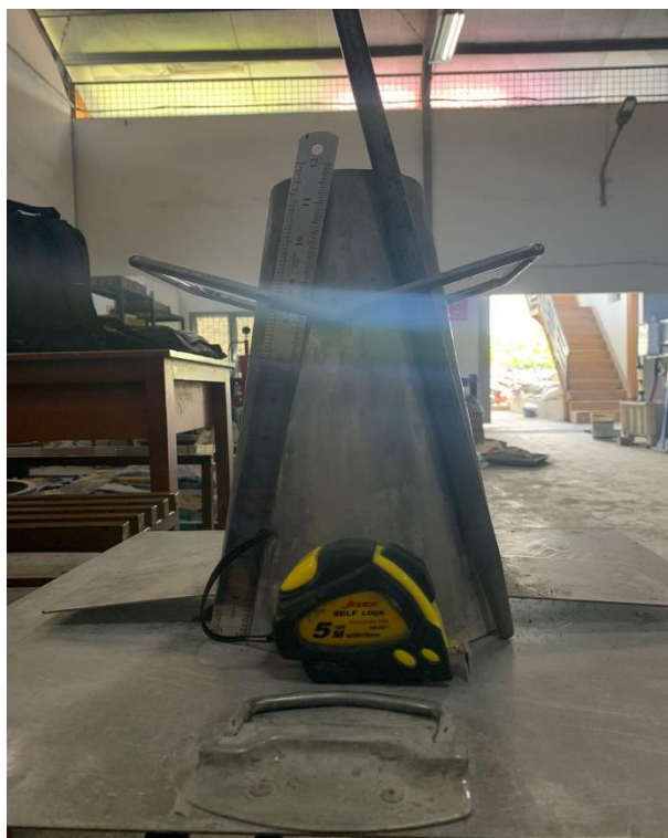
Gambar Lampiran- 14: Satu set alat slump test.
