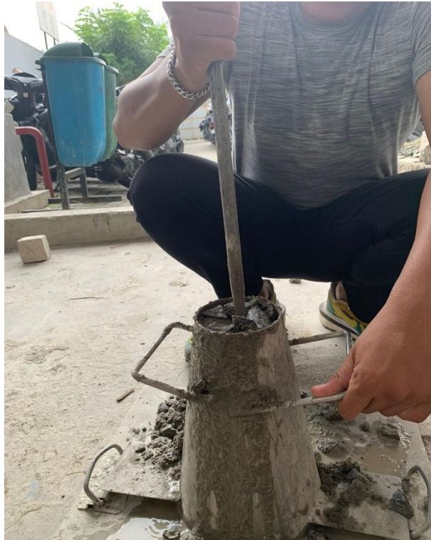
Gambar Lampiran- 31: Slump test.
