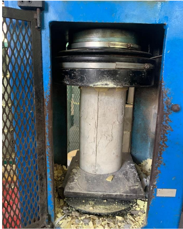
Gambar Lampiran- 35: Model kehancuran beton
