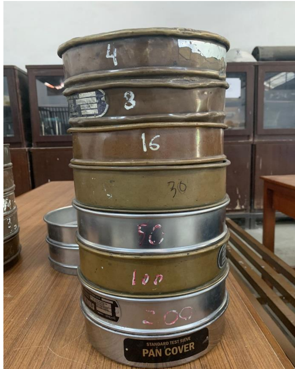
Gambar Lampiran- 7: Saringan agregat halus.
