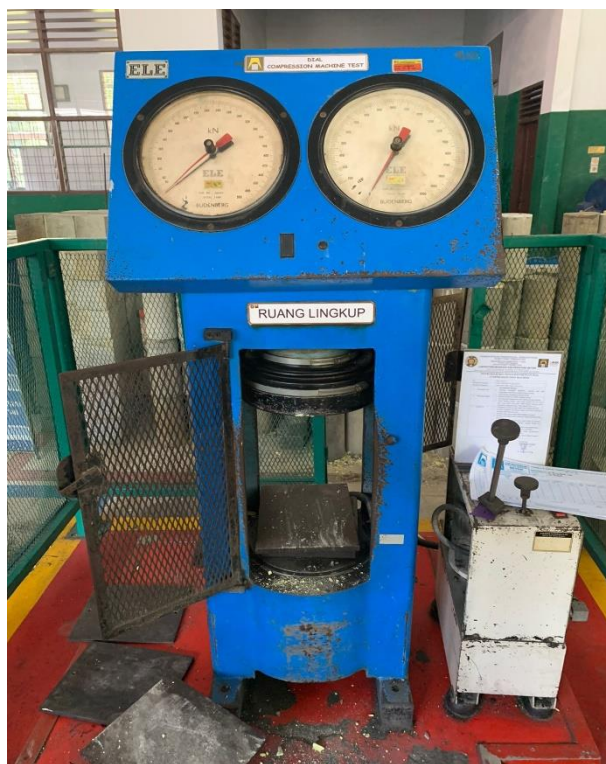
Gambar Lampiran- 25: Compression machine test.
