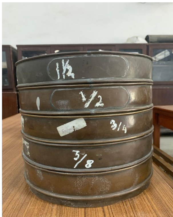
Gambar Lampiran- 8: Saringan agregat kasar.
