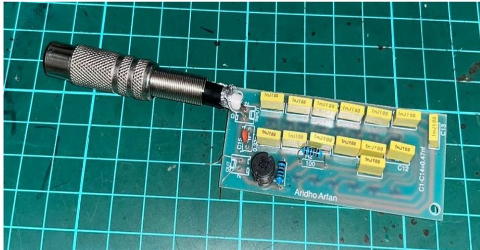
Gambar 4. 11 Prototype RF Harvesting Energy
