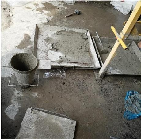
Alat slump test
