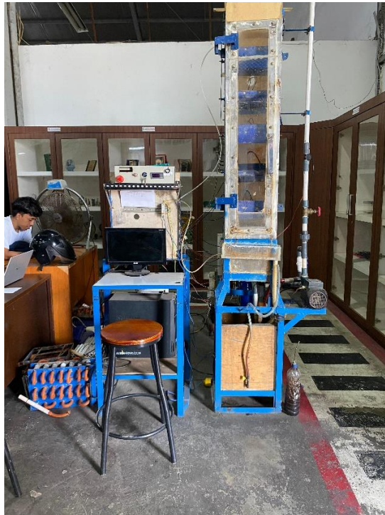
Gambar 3. 1 Prorotipe Cooling Tower
