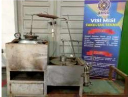
Gambar 3.5 Mesin Pirolisis Laboratorium UMSU
