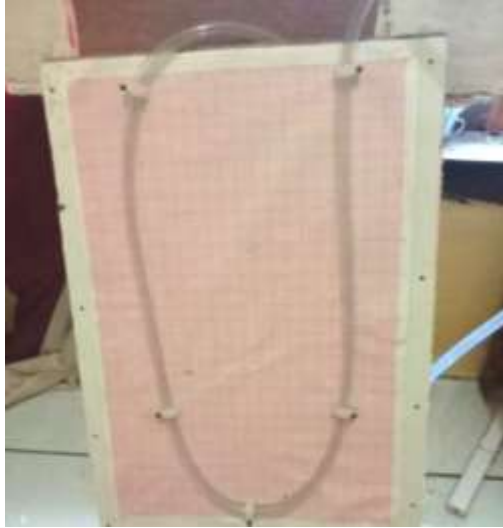
Gambar 3.9 Manometer tipe U Selang 5 mm
