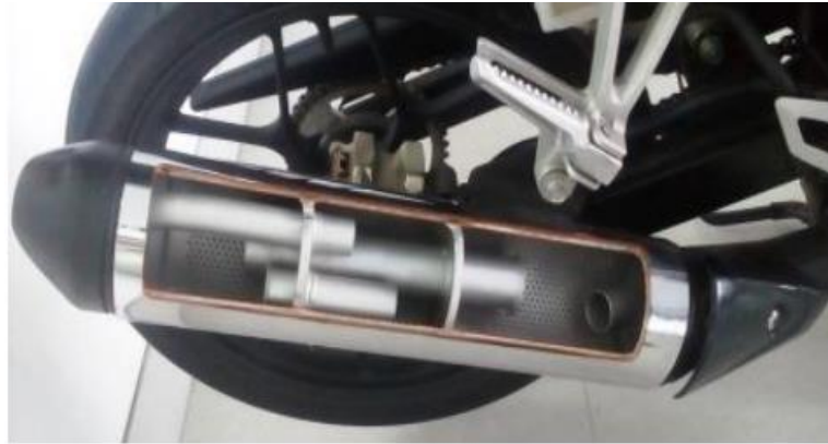
Gambar 2.2 Resonator Knalpot.(A. Graham Bell. Haynes publishing)
