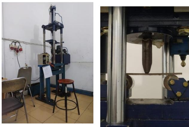
Gambar. 3.35 Setup alat uji *Three Point Bending*
