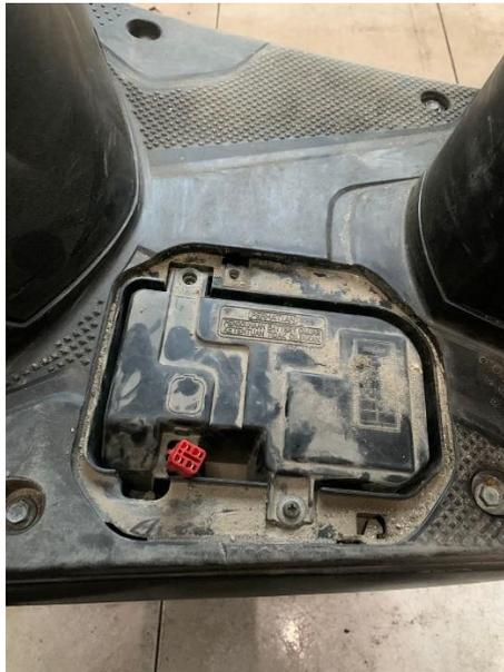
Gambar 3.22 Socket *DLC* ( data link conector)
