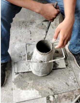
Gambar L.12: Proses Uji *Slump Test*
