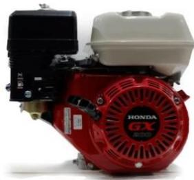
Gambar 2.12 Motor Penggerak (Fadli, 2015)
