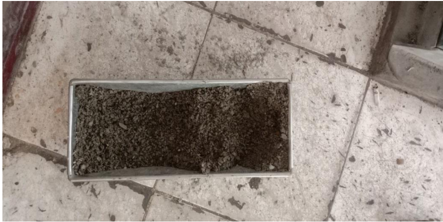
Gambar L.5: Agregat Halus FA
