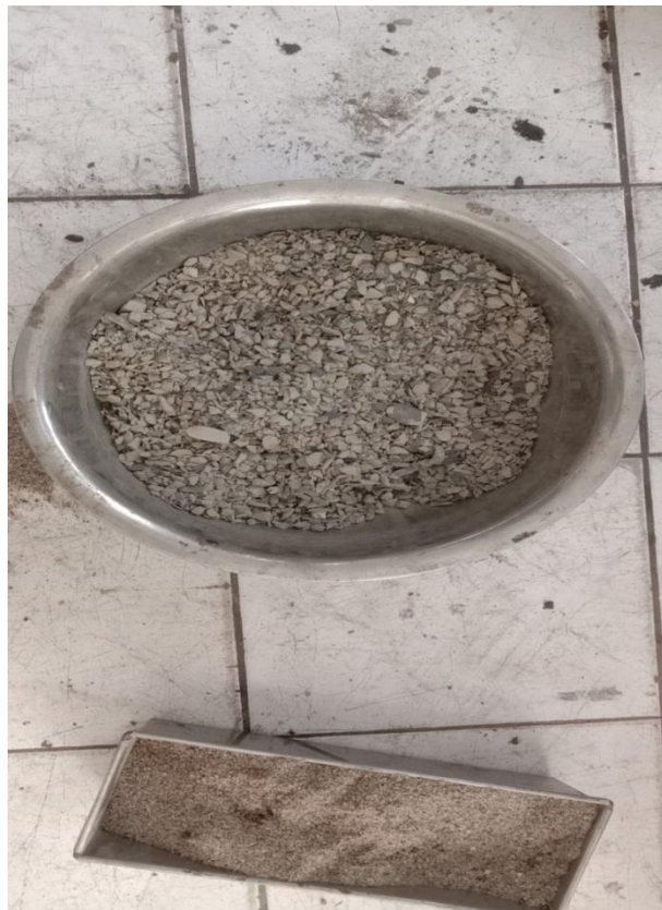
Gambar L.4: Agregat Kasar MA 1/2 inch
