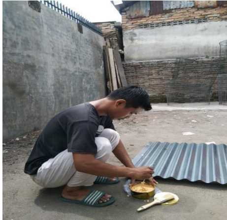
Gambar 3.14 Pengolesan Wax Mirror Glaze
