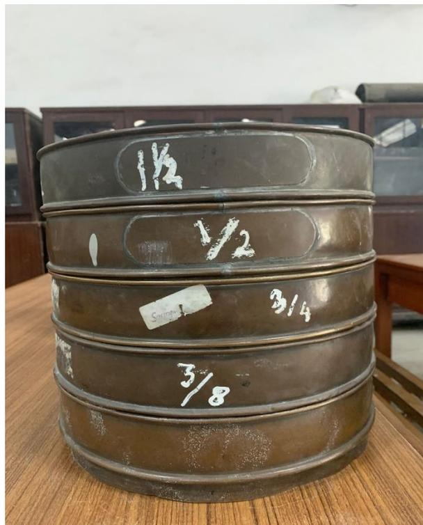
Gambar Lampiran- 8: Saringan agregat kasar.
