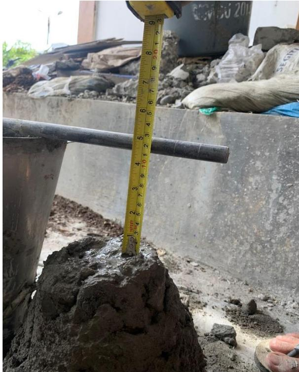
Gambar Lampiran- 31: Slump test.
