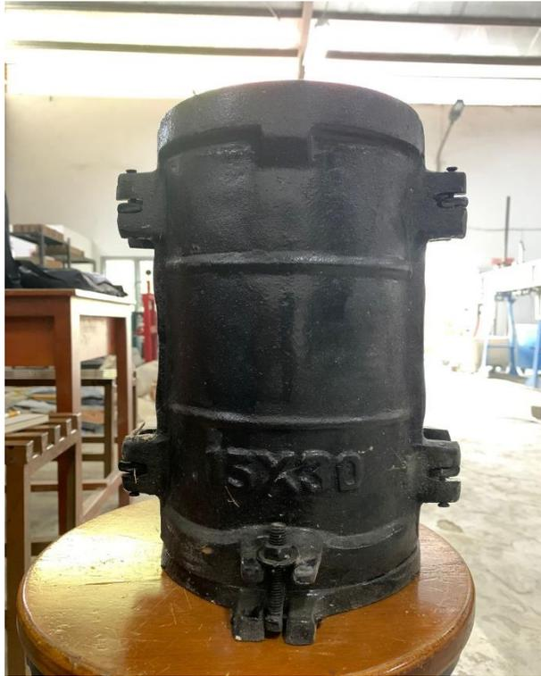
Gambar Lampiran- 19: Cetakan Silinder.
