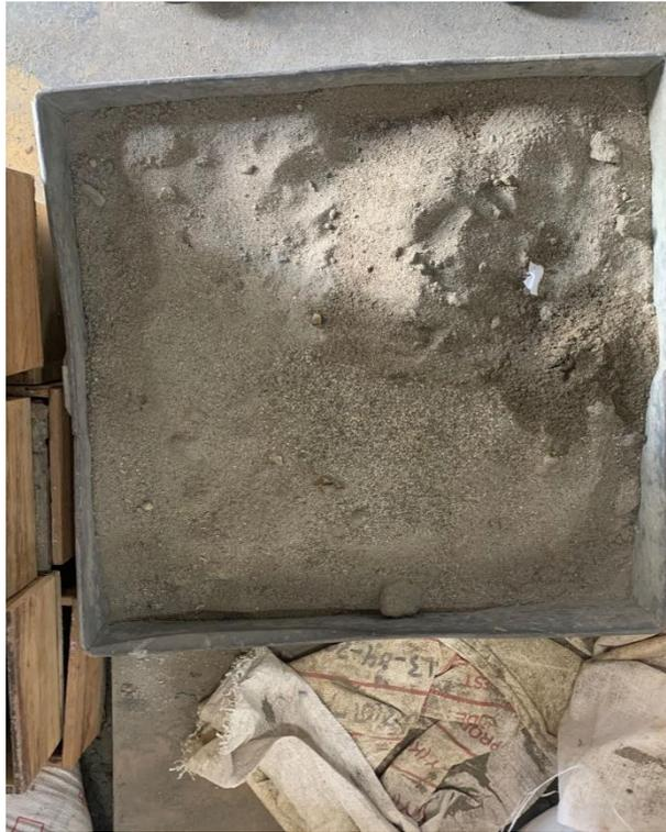
Gambar Lampiran- 3: Agregat halus.
