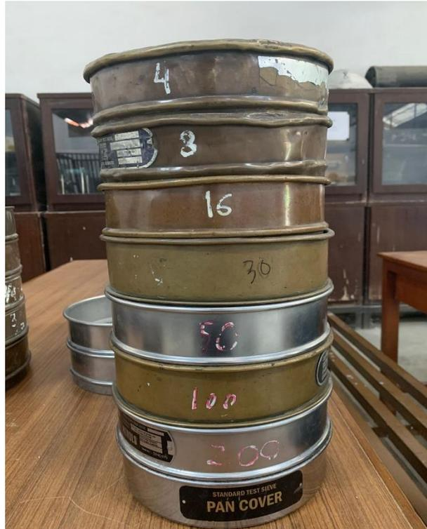
Gambar Lampiran- 7: Saringan agregat halus.
