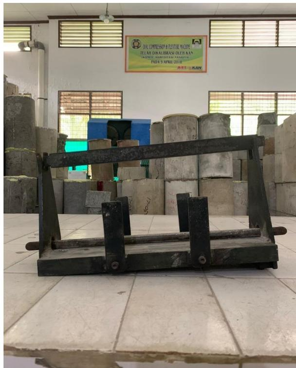
Gambar Lampiran- 36: Alat bantu perata beban (Keranjang beton).
