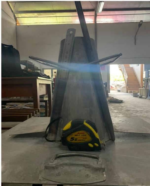
Gambar Lampiran- 14: Satu set alat slump test.
